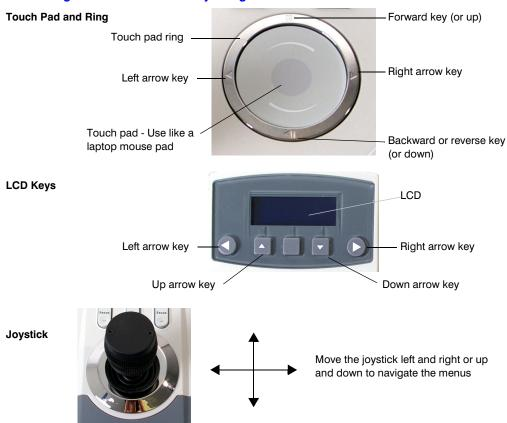
Figure 2-2 The UltraKey Navigation Controls
